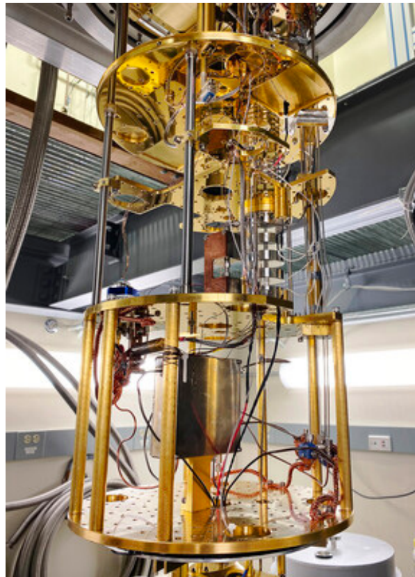
Experimental electronics in the dilution refrigerator. These components ensure that quantum noise dominates the experiment.
